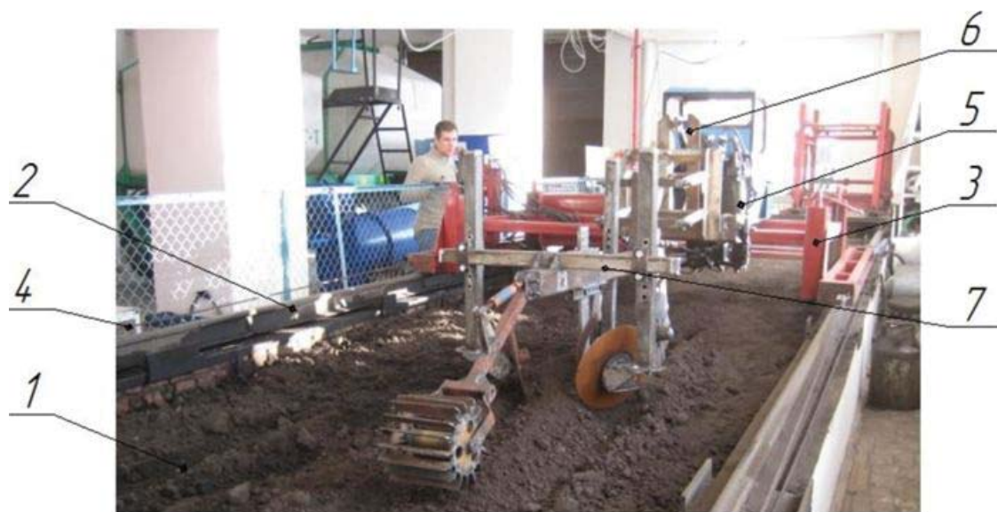
Figure 1: Laboratory unit for determining traction resistance. 1 - tillage bin sized 3x15m; 2 - rails; 3 - powered bogie; 4 - MIC-400D analog to digital converter; 5 - strain-measuring hinge with sensors; 6 - hydraulic system; 7 - developed cultivator gang for strip-till planting
